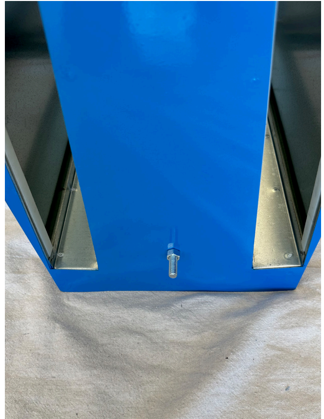
Figure 2H. Install door latch hardware
