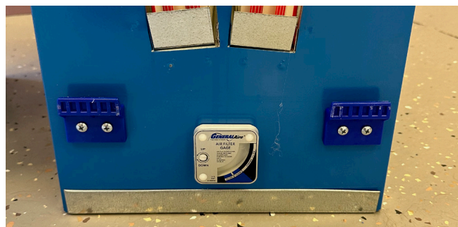
Figure 6J. Install filter gauge.
