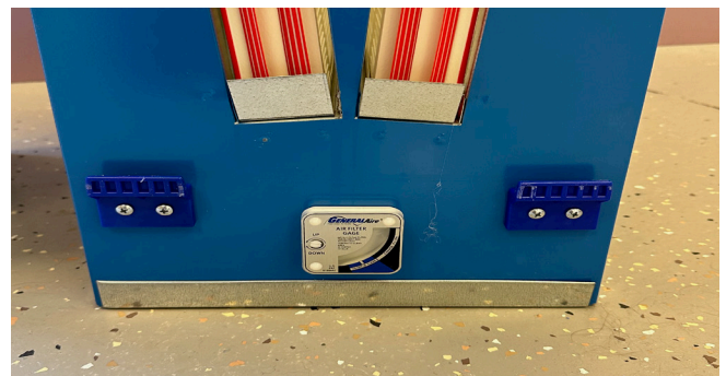
Figure 2J. Install filter gauge
