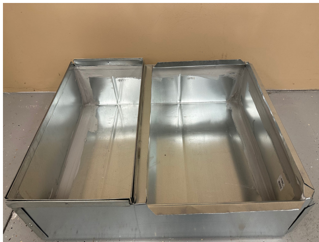
Figure 6C. Build/use a Prefab furnace base. Seal the base.
