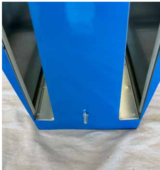
Figure 1G2. Install the door latch hardware.
