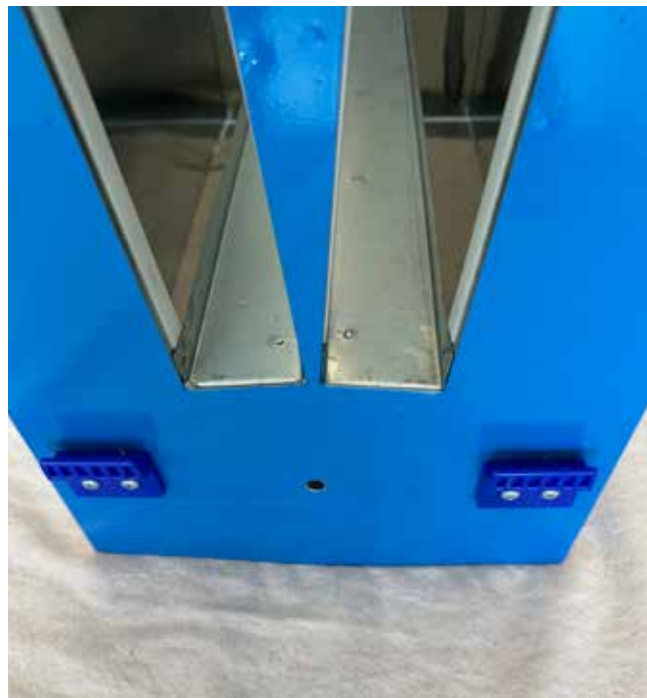
Figure 1G1. Install the door mounting hardware.
