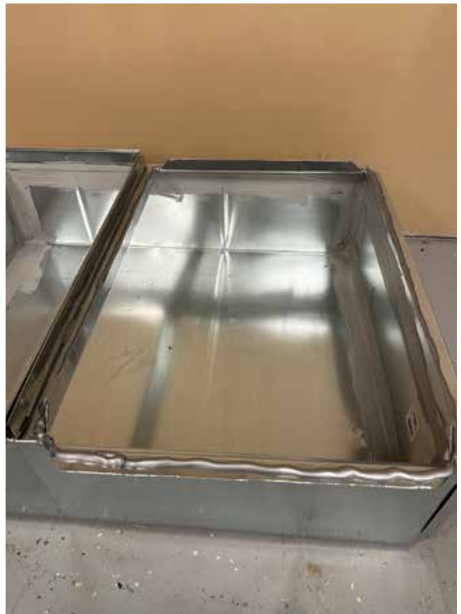
Figure 6D1. Put sealant on connecting surfaces.
