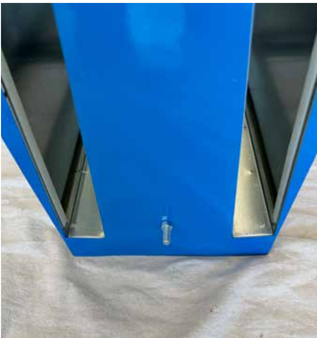
Figure 3F. Install door latching hardware.
