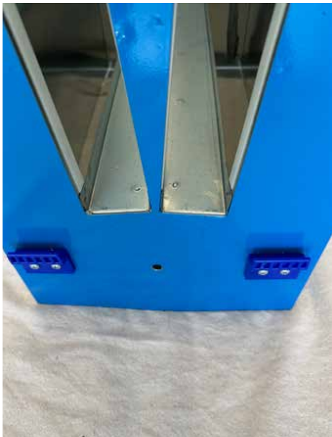
Figure 2G. Install door mounting hardware
